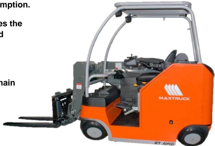
Electric four wheel forklift with Omni-directional drive make it easy to handle long loads (6m) and bulky loads without any risk for accident or damages on equipment, load or personal in vicinity.
